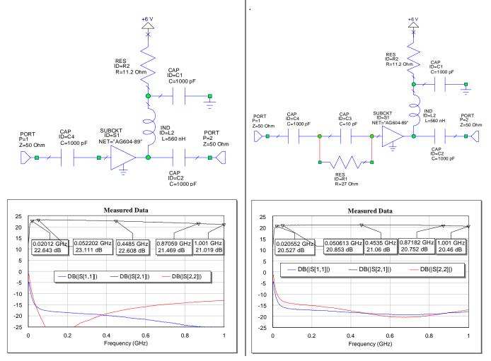
In both examples shown above, a 560 nH inductive RF choke was used. To decrease the gain rolloff and degraded return loss performances at lower frequencies below 40 MHz, a larger inductance value is recommended. This is due to the fact that the impedance the RF choke presents to the circuit is only 70  $\Omega$  ( $Z = j\omega L$ ) at 20 MHz.
